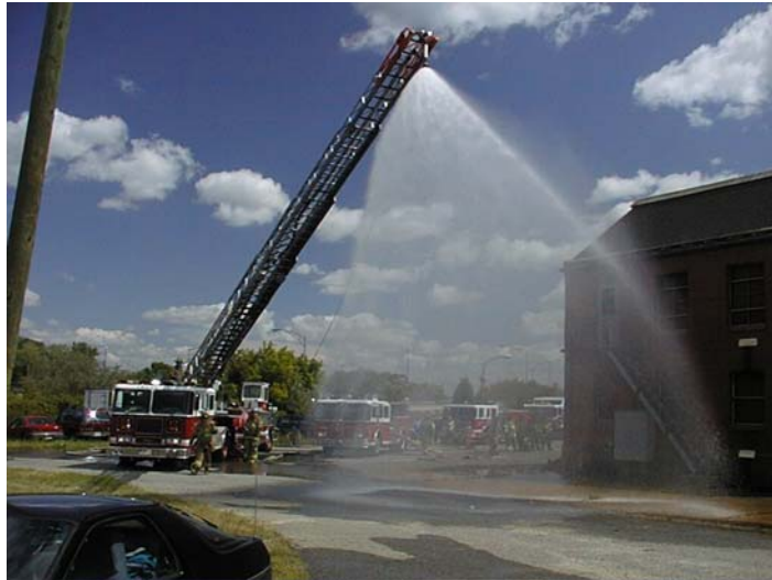
Figure 4-1. The Ladder Pipe Decontamination System
