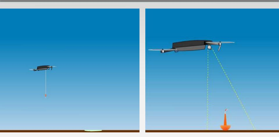
Demonstration of remote sampling: UAV immerses a piece of indicator paper into a "chemical spill" to result in a colour change
