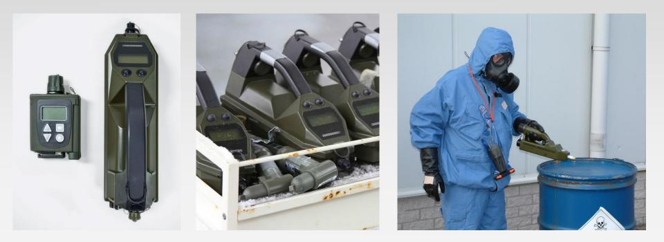
A single response by a detector (or CALID paper colour change) is only an indicator of the presence of a Schedule 1 chemical agent
