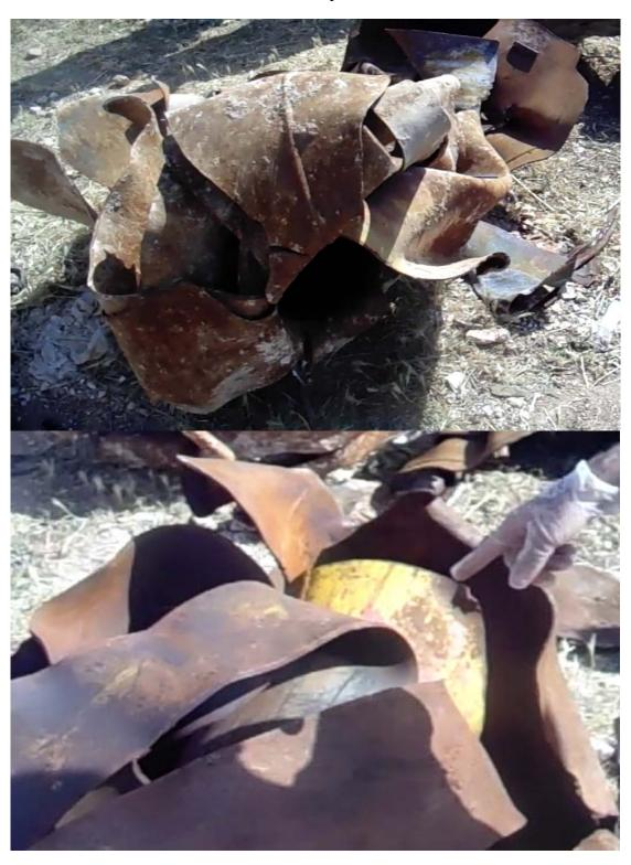
The remnants of a toxic chemical cylinder. Note that the cylinder has ruptured at the nose end.
