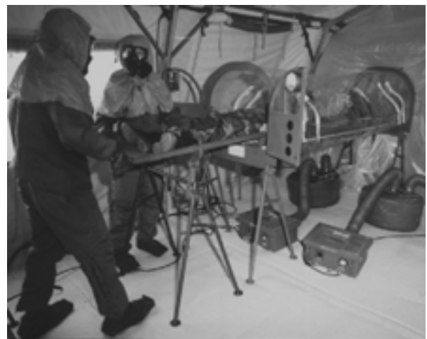
Fig. 16-34. The litter-patient airlock of the Chemical and Biological Protected Shelter. Treating casualties on a chemical-biological warfare battleground requires complicated procedures, even to get the casualty into a protected environment for examination. Special air locks for casualties and new procedures had to be developed. Photograph: Courtesy of Chemical and Biological Defense Command Historical Research and Response Team, Aberdeen Proving Ground, Md.
