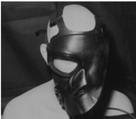
Fig. 16-2. The M45 protective mask facepiece has two skins. The inner skin is composed of silicone rubber, and the outer skin is composed of butyl rubber. This arrangement maximizes both mask-to-skin seal and chemical agent impermeability. A similar design is used in the M40 protective mask. Photograph: Courtesy of Visual Information Division, US Army Chemical and Biological Defense Command, Aberdeen Proving Ground, Md.
