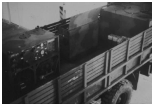
Fig. 16-41. The M12A1 Power-Driven Decontamination Apparatus (PDDA).
