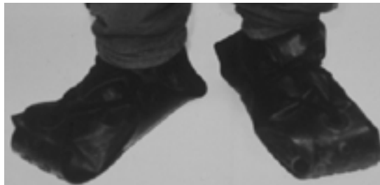
Fig. 16-16. The chemical protective footwear cover (CPFC).
