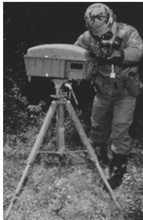
Fig. 16-30. Field use of the M21 Remote Sensing Chemical Agent Alarm (RSCAAL). Reprinted from Brletich NR, Waters MJ, Bowen GW, Tracy MF. Worldwide Chemical Detection Equipment Handbook . Edgewood, Md: Chemical Warfare/Chemical and Biological Defense Information Analysis Center; October 1995: 425. Photograph: Courtesy of Brunswick Corporation (now Intellitec), DeLand, Fla.
