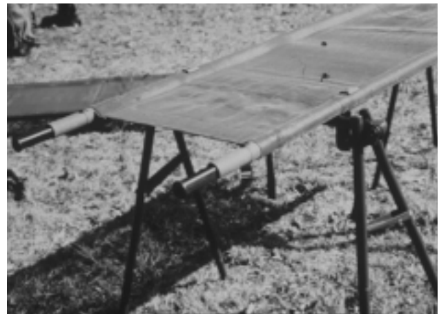
Fig. 16-43. The decontaminable litter.
