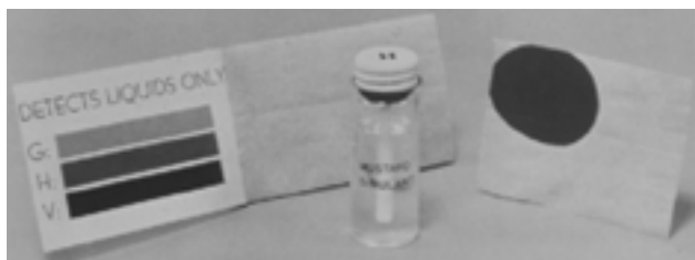
Fig. 16-24. M8 Chemical Agent Detection Paper. A drop of mustard (H) simulant from the vial has turned the paper red. Reprinted from Brletich NR, Waters MJ, Bowen GW, Tracy MF. Worldwide Chemical Detection Equipment Handbook . Edgewood, Md: Chemical Warfare/Chemical and Biological Defense Information Analysis Center; October 1995: 407. Photograph: Courtesy of US Army Edgewood Research, Development, and Engineering Center, Aberdeen Proving Ground, Md.
