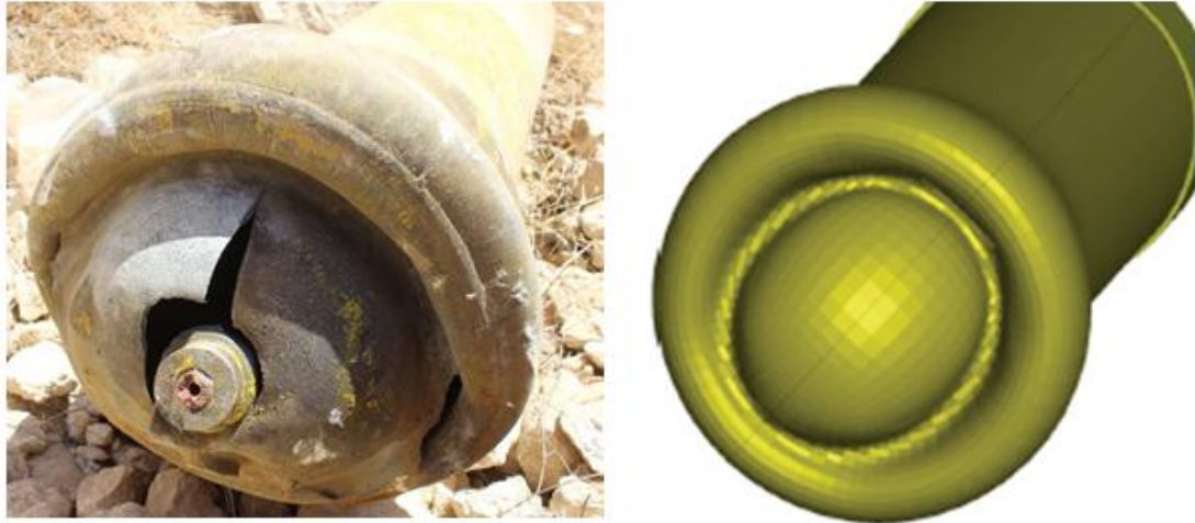
FIGURE 16: PHOTOGRAPH OF THE CYLINDER'S HEAD TAKEN ON 2 OCTOBER 2016 (LEFT). SIMULATED IMPACT OF THE CYLINDER EQUIPPED WITH A NOSE CAP AND IMPACT VELOCITY OF 120 M/S ONTO TERRAIN SLOPED 20° FROM PERPENDICULAR (RIGHT)
