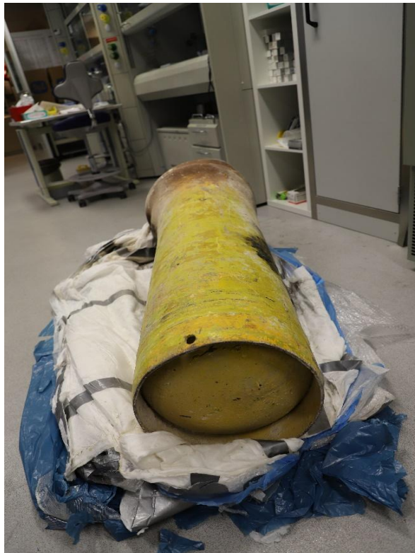
FIGURE 10: BASE OF THE RECOVERED CYLINDER
