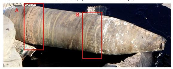
7.52 The condition of the rotating band (Figure 8-A) and bourrelet (Figure 8-B) indicate that the projectile had been fired.
