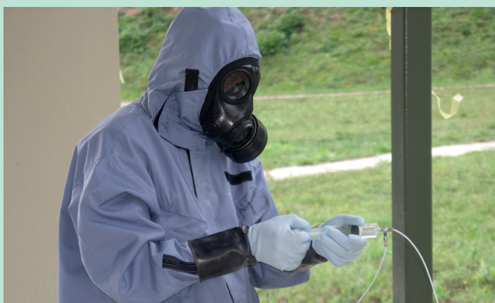
Figure 2. An inspector collecting a liquid sample during and challenge inspection (CI) exercise
