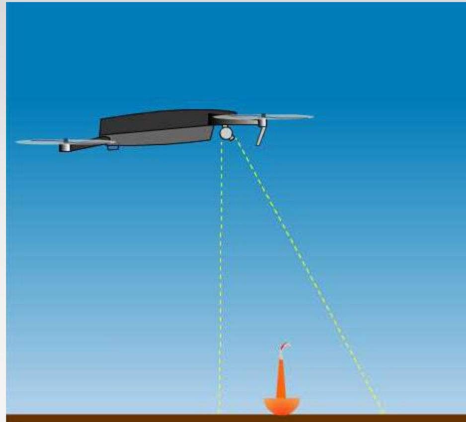
**Demonstration of remote sampling: UAV immerses a piece of indicator paper into a “chemical spill” to result in a colour change**
