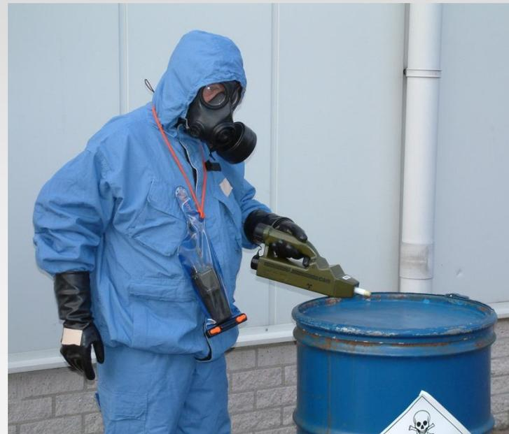
**A single response by a detector (or CALID paper colour change) is only an indicator of the presence of a Schedule 1 chemical agent**
