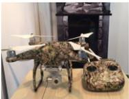
Lightweight drone with visible imaging camera payload. Photograph by Wesam Alwan
