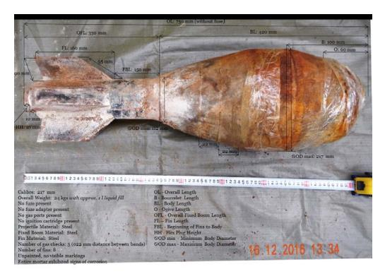
Picture 9. Photograph of the mortar with dimensions and description.
