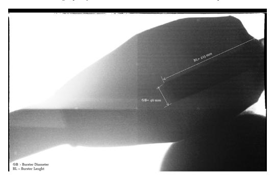
Picture 10. X-Ray image of the mortar indicating the liquid level and internal burster dimensions.
