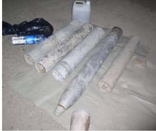
Figure 2: Canister placed in barmine stack. Further barmines were then placed over the “lid” and donor charges and initiators fixed.
