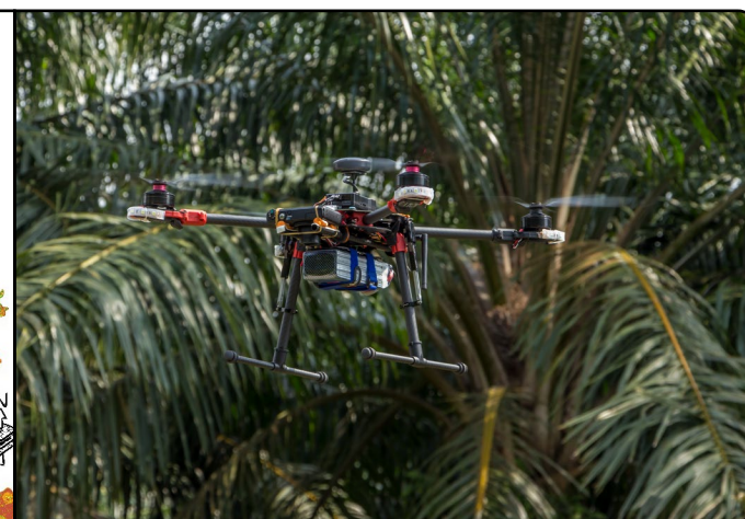
A drone equipped with Near Infrared sensors and Cloud access. Image by Cesar Harada
